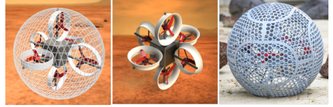
Figure 1: Left: Rollocopter concept art, including propellers, electronics (gray box) and the impact-resilient cage. Middle: hexacopter configuration of the propellers. Right: A Rollocopter prototype. The spherical cage allows to roll on flat terrains and to be impact-resistant, while the configuration of the propellers guarantees actuation in any direction.
