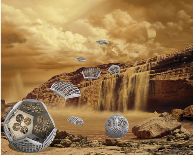
Figure 2: Artist's representation of the Shapeshifter [8] platform self-assembling to the Rollocopter shape. The Shapeshifter is a multi-modal and multi-agent platform for the exploration of planets and their moons with an atmosphere, such as Titan.
